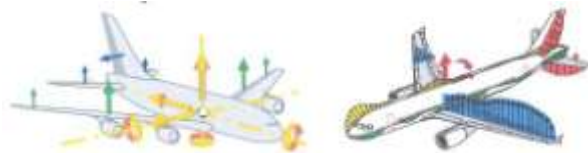
Relevant aerodynamic information for computational flight testing: forces and moments (left), and surface pressure distribution (right)
