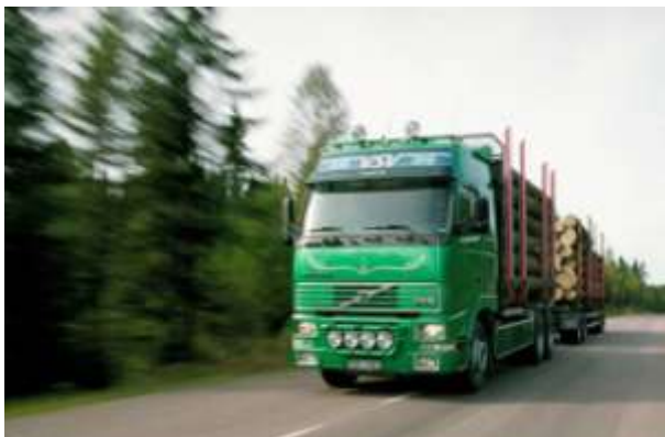
Figure 1: Transport vehicles are exposed to dramatically different conditions in different parts of the world and different transport missions. The timber truck needs to sustain very high pay loads, as well as high dynamic loads.
