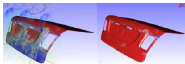
Figure 2: Painting a trunk lid. Colors on the surface show the film thickness with blue being un-painted and red a film thickness of at least 100 \mu\text{m} after 3 s (left) and 6 s (right). (Geometry courtesy of Saab Automobile).
