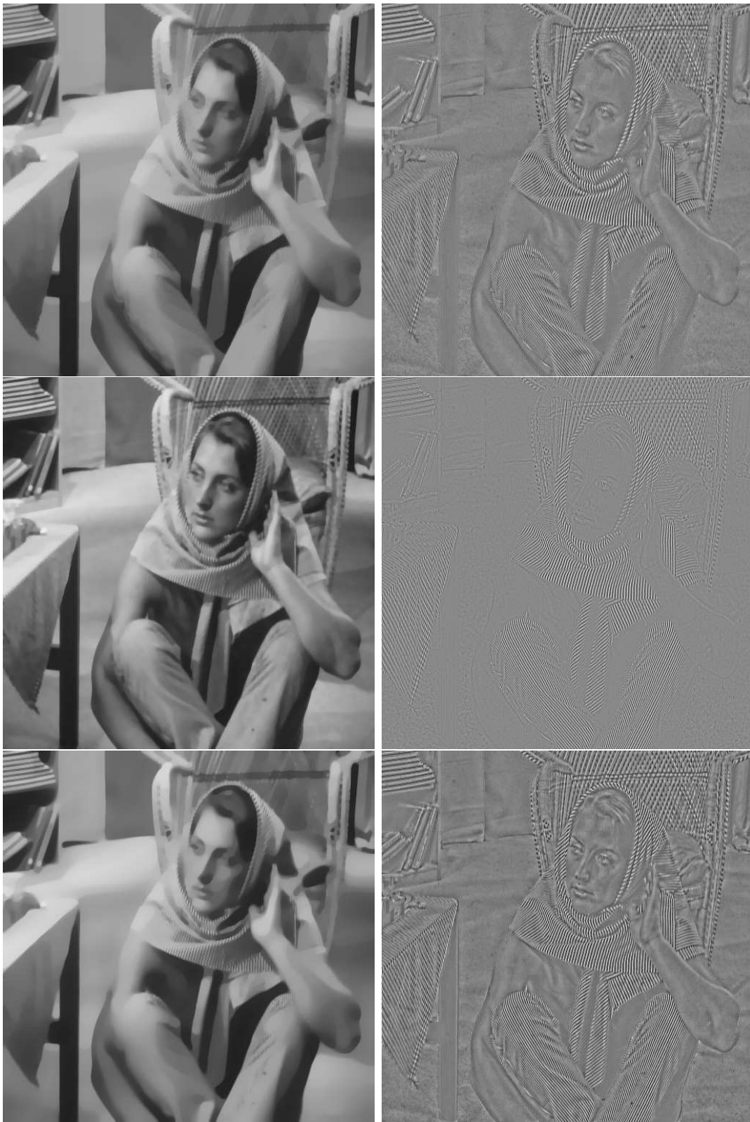
Figure 3: TL : Cartoon part for ROF model - TR : Texture part for ROF model - ML : Cartoon part after 4 seconds - MR : Texture part after 4 seconds - BL : Cartoon part after 5 minutes - BR : Texture part after 5 minutes
