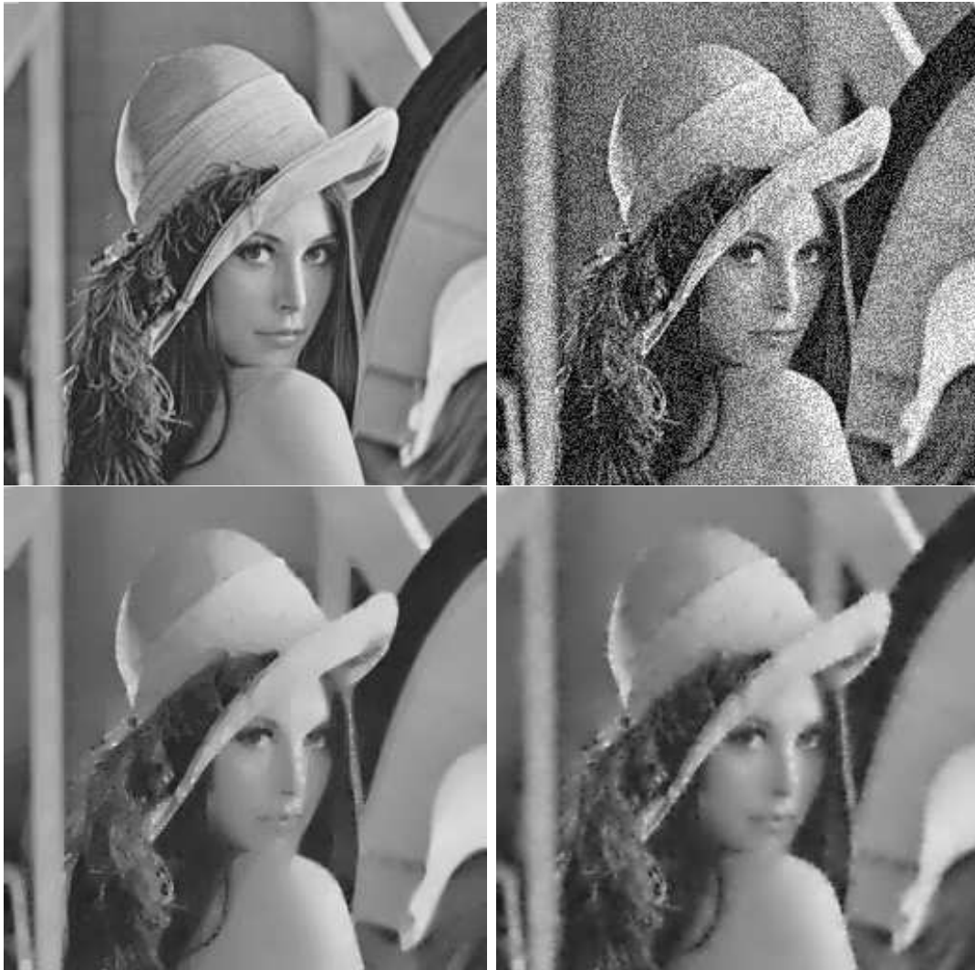
Figure 4: TL : lena image on [0, 1] - TR : lena image + U([-0.2, 0.2]) BL : Denoised with BV - L^\infty BR : Denoised with MinSurface - L^\infty
