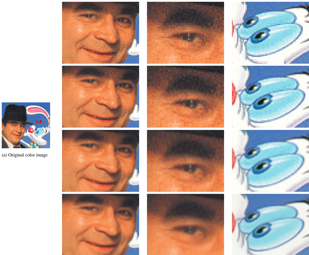
Figure 7: Comparisons of image resizing, using Nearest-neighbor (first row), Linear (second row), Bicubic (third row) and PDE-based (last row) interpolations.
