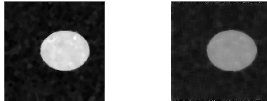
1- Median filter \Delta B = 94.8\% \Delta N = 96\% 2- Despeckle with The Gimp \Delta B = 95\% \Delta N = 85\%
